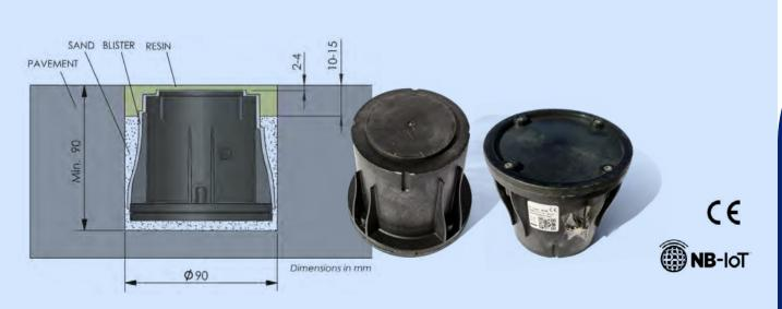
Higher than 98% **Accuracy** Sampling rate Every 3 seconds Connectivity LTE band 8 (NB-IoT) **Power supply** Autonomous through battery **SIM Card** SIM on chip (MFF2) **Battery Life** Up to 10 years (under standard coverage quality of the mobile network) **Dimensions** Height: 8.3cm, Base Diameter: 9.5cm by 6.8cm at the top Weight 345 grams **Ingress protection** IP68 (completely sealed housing)IK10 **Pressure resistance** 1.5 Tons **Operating temperature range** -33°C a 65°C
